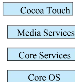
Figure 2.17 Architecture of Apple's iOS.
